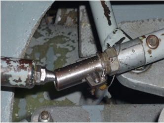
Standard L'Hotellier connection with locking pin
